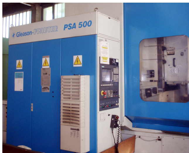
Photo: Gleason Pfauter PSA 500 Gear shaping with DiaGrind 535/15
