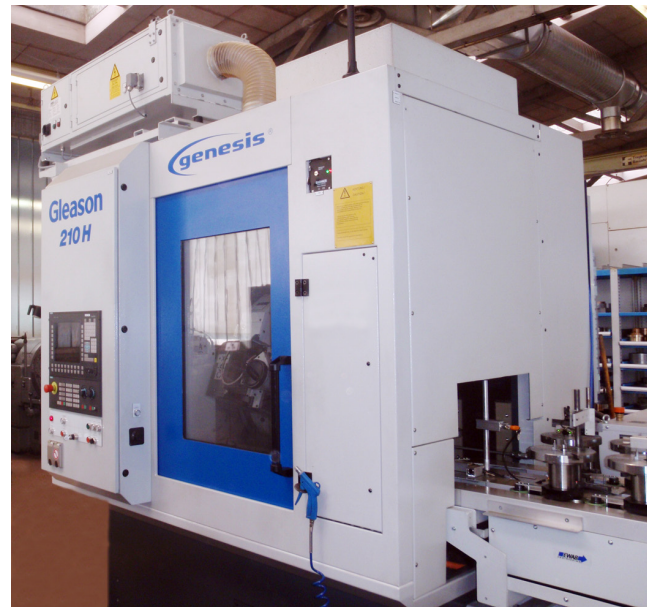
Photo: Gleason Pfauter 210 H Genesis Gear hobbing with DiaGrind 535/15
